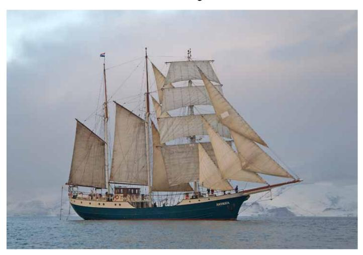
The SV *Antigua* was built in 1957 in Thorne (UK) and served for many years as a fishing vessels, until it was completely re-built in the early 1990s in the Netherlands as a barkentine and equipped as a passenger ship. A barkentine has three masts with square sails on the foremast.
